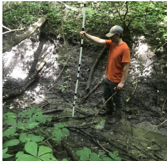
Mark Jacobs collecting stream and channel data needed for design of grade control and bank stabilization measures.
